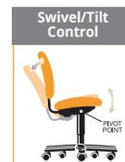
Places the "pivot point" directly above the base center and allows the user to lean back in a seated position.
